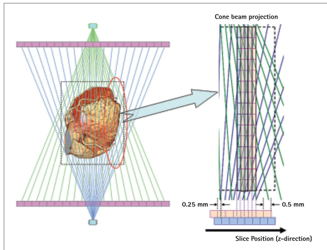
In order to avoid increased patient exposure the coneXact™ reconstruction algorithm is a viable alternative to FFS for improvement of spatial detectability with concurrent avoidance of structural artefacts. We performed phantom test validation to confirm the utility and clinical potential of this reconstruction algorithm in cardiac CTA.
